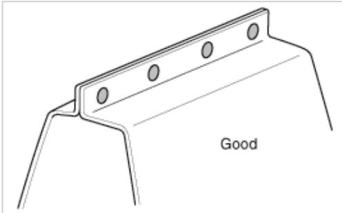
b. Do not weld on the edge of the flange joint.
