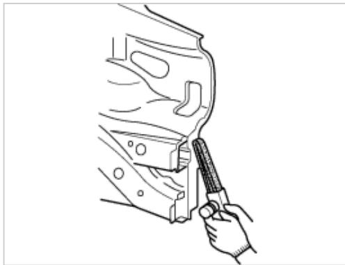
5. Drilling a hole for plug welding
